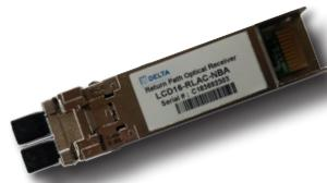
The SFP has a very low power consumption, achieves a very high return path receiver density and it is compatible to DOCSIS 3.1 upstream.
